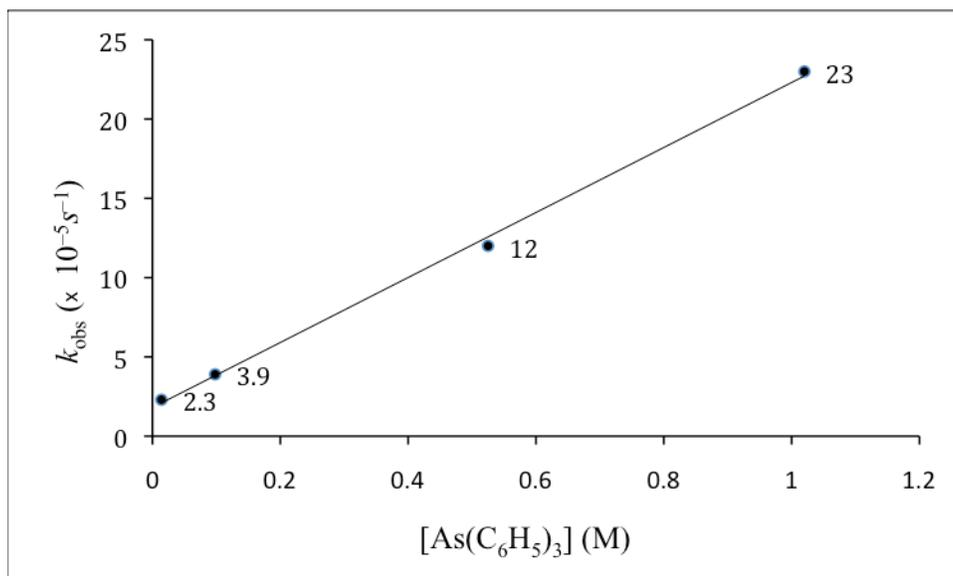
$$\text{Rate} = (k_1 + k_2[\text{As}(\text{C}_6\text{H}_5)_3])[\text{Co}(\text{NO})(\text{CO})_3]$$
